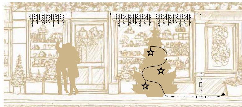
EXAMPLE OF MIXED 230V AND 24V WIRING
